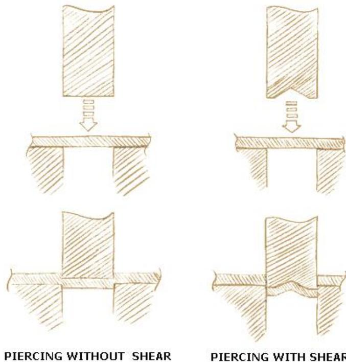
The Punching Force calculated above is multiplied by a shear factor, which ranges in value from 0.5 to 0.9 depending on the material, thickness, and shear depth. For shear depths of 1.5 mm (0.060 in) the shear factor ranges from 0.5 (for 1.2 mm / 0.047 in stock) to 0.9 (for
